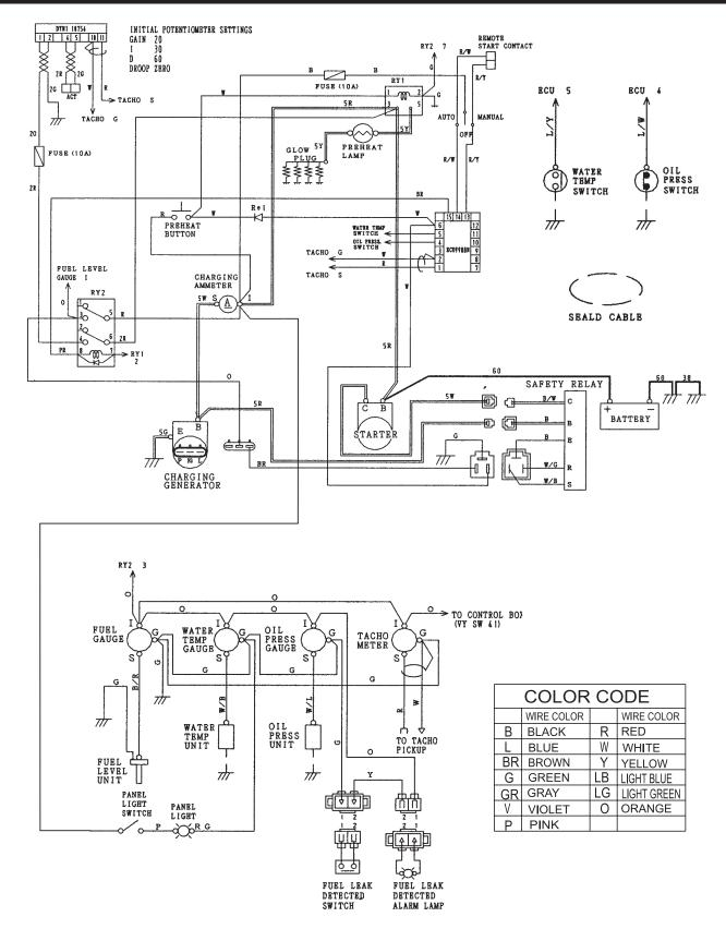
Figure 62. Engine Wiring Diagram
